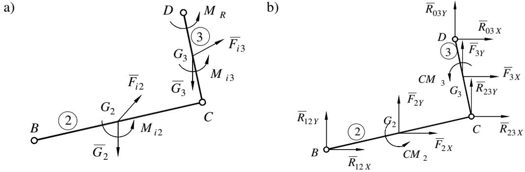
Fig. 3. **Dyad RRR(2, 3)**: a – highlighting forces and moments acting on elements of dyad; b – kinetostatic scheme of dyad
