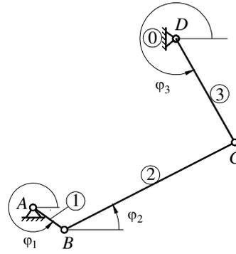
Fig. 2. Defining position kinematic parameters of mechanism
