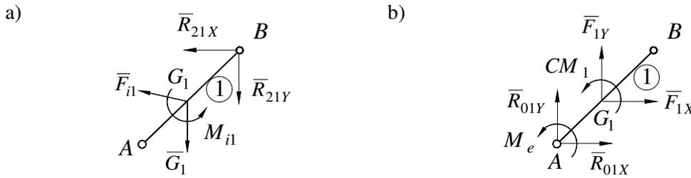
Fig. 4. **Motor group R(1)**: a – highlighting forces and moments acting on elements of group; b – kinetostatic scheme of motor group
