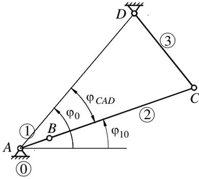
Fig. 1. Defining initial position of mechanism
